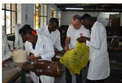
Thermoforming of milled models with 3D cad/cam technology
