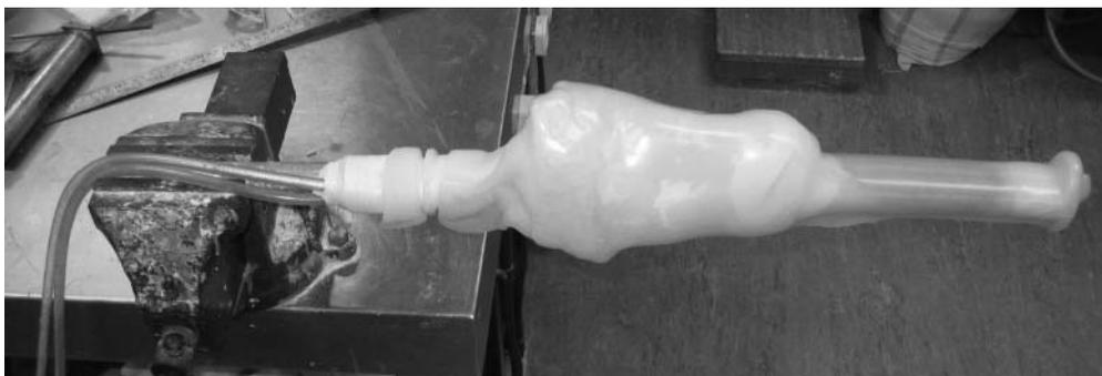
Figure 2. A thermoplastic material sheet is heated and vacuum formed over the entire structure of the foot adaptor, residual limb and pylon mould.
